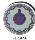
Gyroscope action ratio adjusting knob 陀螺仪作用比调节
