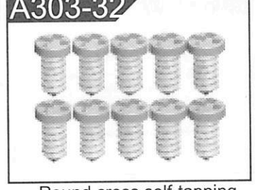
A303-32 Round cross self-tapping ST1.7 * 6 PB D3 black zinc plating components
