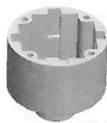
Front differential gearbox
